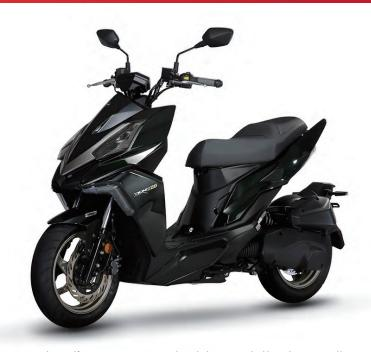
The auto-dimmer LED dashboard that usually found on automobile is adopted for the first time by SYM on DRG to enhance rider's vision scope at night and provides better safety protection. This 158cc scooter of top-notch performance also features a water-cooled engine that combines Z.R.S.G (Zero-Resistance Starter & Generator), 11.4kW/8,000rpm horsepower, peak torque of 15.1Nm/5,500 rpm and economic fuel-consumption of 42.km/L.
