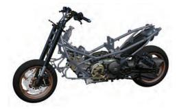
➤ In addition, the 50/50 balanced weight distribution, shortened wheelbase and extended aluminum swing arm make TL born to be excellence at handling, fulfilling both ways of high speed stability and remarkable urban agility.
